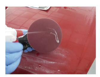
**5. Bodyshine Application** Use the 2000 grit Blend and Finish to remove the P1500 scratches.
