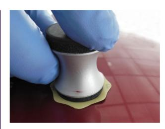
3a. Small Area Inclusion Removal For small isolated dirt inclusions, use the denib block with the denib abrasive disc. Top Tip—use the Bodyshine to lubricate the abrasive.
