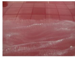
4. Sanding Area Check all the dirt inclusions have been removed and wipe the dust away.
